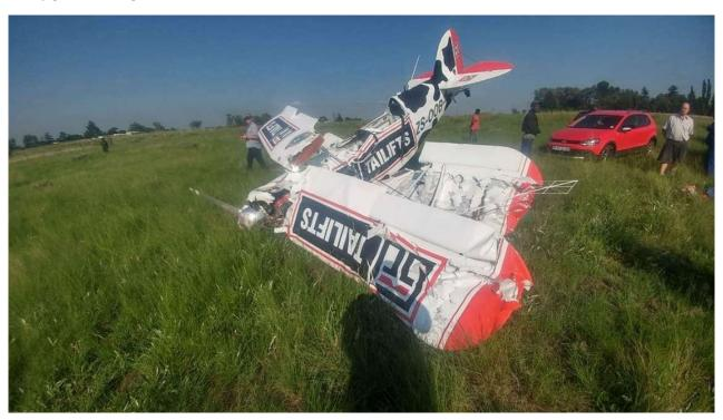
The cause of this excitement? The conrod bolts sheared and the broken bolts went through the crankcase. The prop stopped dead. Sounds alarmingly like a previous conrod-cylinder smashing event that also resulted in a forced lob into the Tugela Valley a few months ago. Wonder if this one was also due to incorrect assembly?
